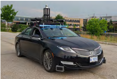
Fig. 1: The Autonomoose research vehicle with the visual signal communication system prototype (S-T signal is ON)
