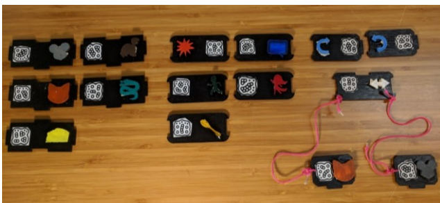
Figure 2. Blocks used in the initial StoryBlocks prototype include characters (mouse, turtle, cat, snake, cheese), actions (explode, talk, run, dance, eat), and control structures (repeat, branch).
