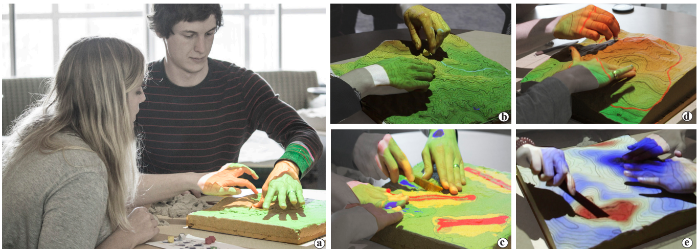
Figure 1: (a) Participants interacting with Tangible Landscape during the pilot study to learn about topographical properties relevant to (b) hydrology; (c) geomorphology; and (d & e) land surface grading.
